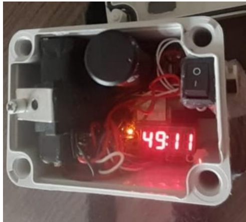
Figure 2. Internal Electronics of the Drone Tracker
