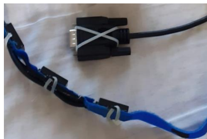
Figure 1. Multi-Level Water Tank Sensor Assembly
