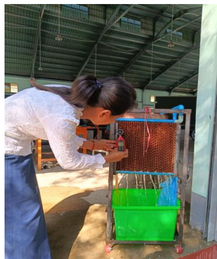
Figure 3. Performance Test of Air Cooler
