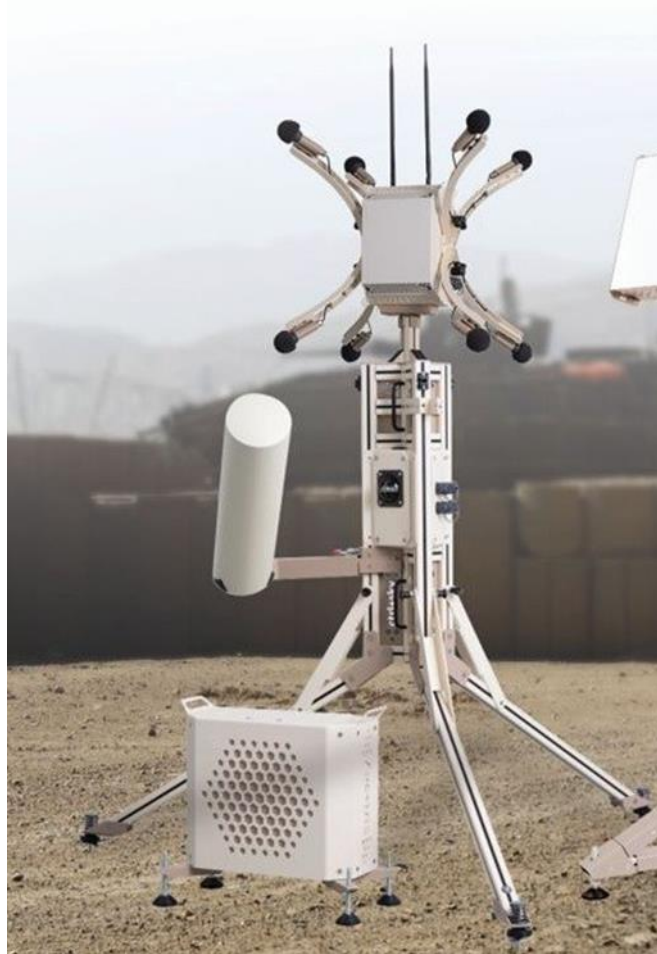
Figure 6. The acoustic sensor of the SKY CTRL antidrone system [19].
