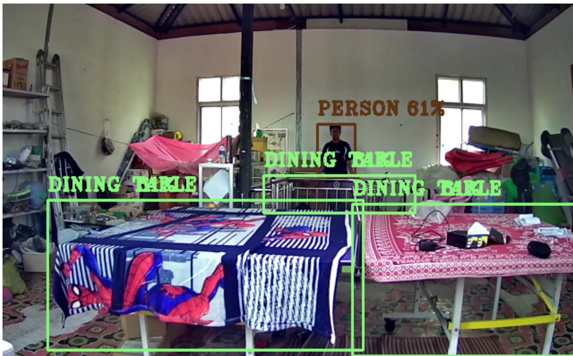
Figure 14. YOLOv8 Object Detection Output(at 25 feet distance)
