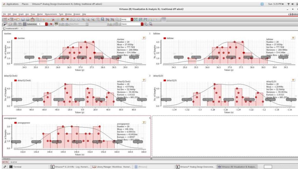
Figure 19. Simulation Results of Rise time, Fall time, Delay, and Average power consumption for DFF-T technique by using Monte Carlo Sampling with ADE-XL simulator
