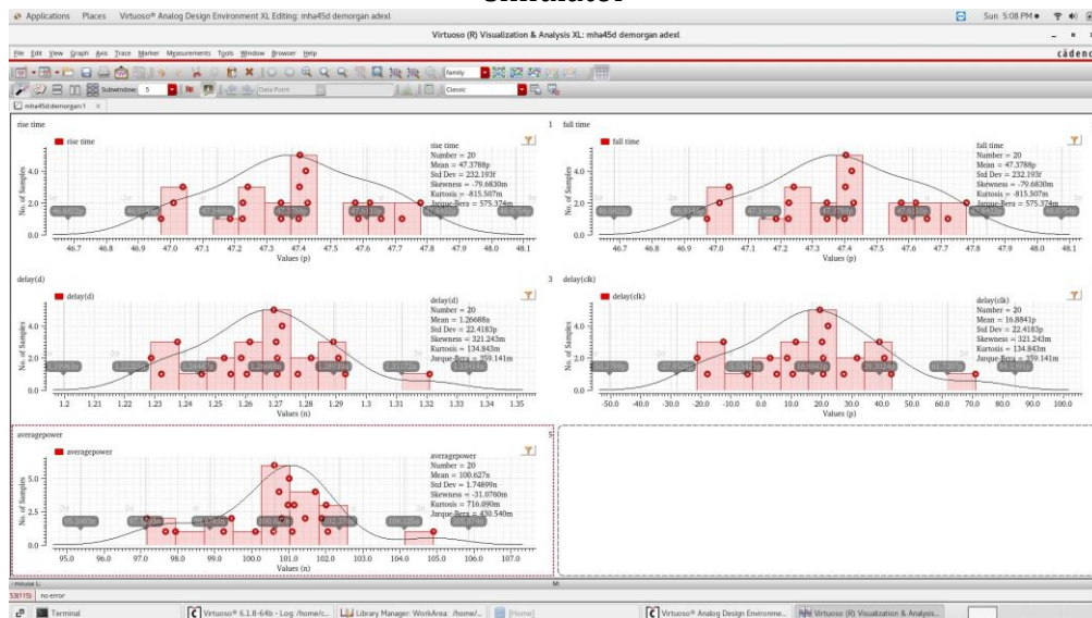
Figure 20. Simulation Results of Rise time, Fall time, Delay, and Average power consumption for DFF-DL technique by using Monte Carlo Sampling with ADE-XL simulator
