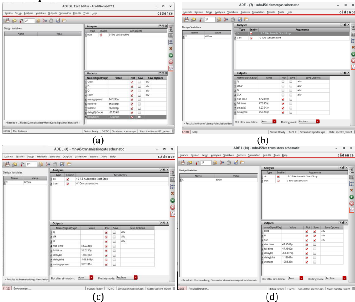
Figure 18. (a) Rise time, Fall time, Delay ,and Average power consumption values for DFF-T technique, (b) Rise time, Fall time, Delay ,and Average power consumption values for DFF-DL technique,
