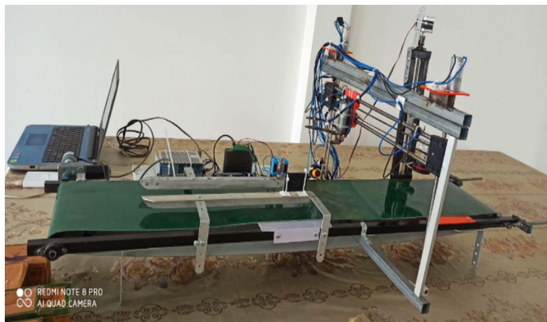
Figure 8. Initial Condition of Stamping Machine
