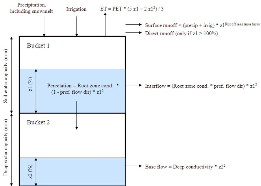
**Figure 2.** The Soil Moisture Method used in WEAP model
